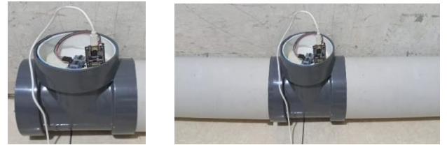
Figure. 5. Implementation HC-SR04 sensor on PVC pipeline connection
