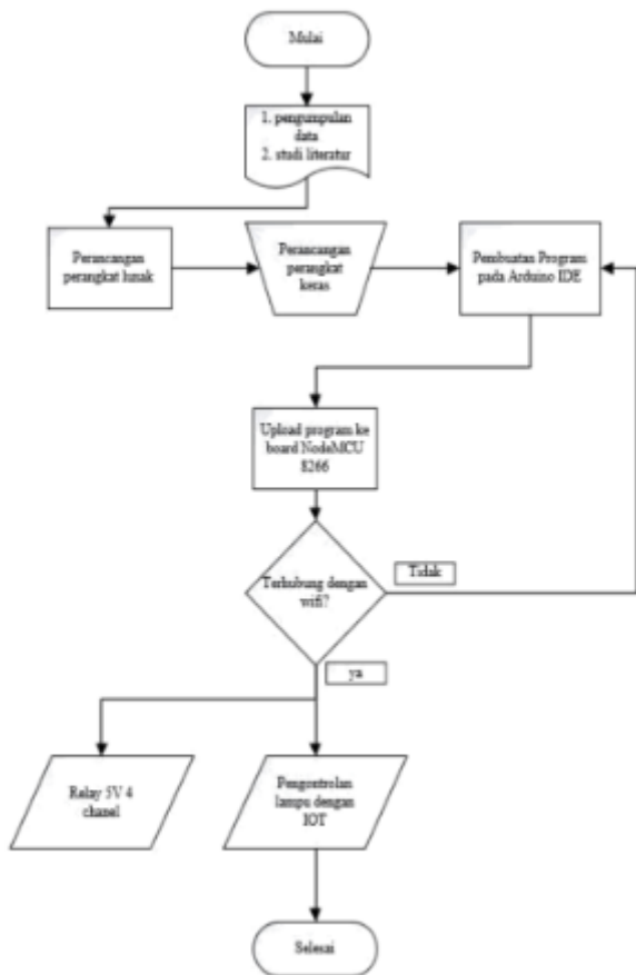
Figure 2. Flowchart of Lighting Control System with IoT
